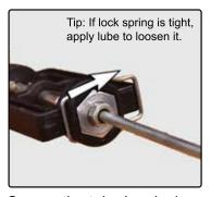
Secure the tube by placing the collet into the hex cavity and sliding the lock spring to the closed position.
