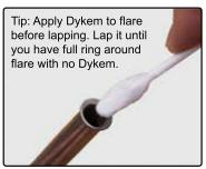
Remove the tube from the Surseat. Clean and inspect the flare for a clean seat. Ready to use.
