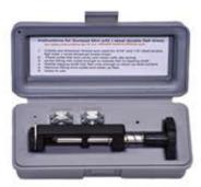
The Surseat P-45 comes with 3/8" x 24 and 7/16" x 24 collets for brake lines with a 45° double flare.
