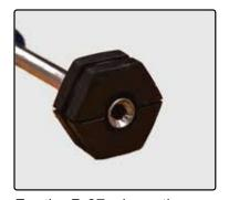
For the **P-37**, clamp the brake line with the appropriate collet size.
