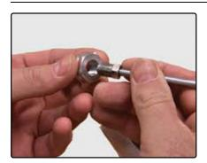
For the **P-45**, screw the fitting into the corresponding collet size for 3/16" or 1/4" tube.
