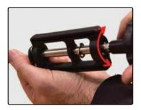
Rotate the lapping head back and forth until a clean seat is formed. More is not better.
