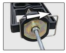
3) Secure the tube in the hex cavity by sliding the lock spring to the closed position.
