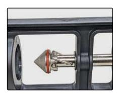
1) Install the lapping heads by pushing them onto the clip. To remove them, lift the clip.
