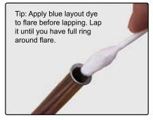
6) Remove the tube from the Surseat. Clean and inspect the flare for a clean seat. Ready to use.
