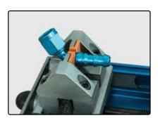
Install angled fittings as shown. Use the plastic inserts to protect anodized fittings. DO NOT OVER TIGHTEN.
