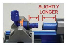
The lenghth of the hose extended from the clamps should be 1/4" longer than the length of the barb so it can be fully installed without hitting the bumper.
