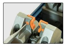
To remove the inserts, use a pin punch or similar as shown.
