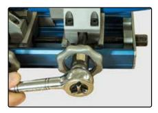
Use a ratchet and 17 mm socket to clamp the hose tighter if necessary.
