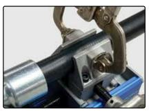
If necessary, use a pair of vise grips for extra clamping force.
