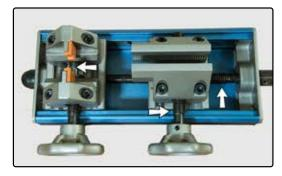
Lubricate the lead screw and threads on the vise wheels with a light oil before using it for the first time and routinely thereafter for trouble-free service.
