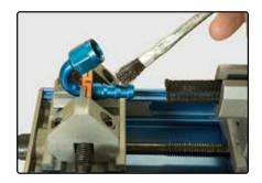
If necessary, lube the barb for easier installation.
