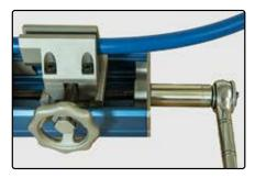
Install the hose with a ratchet, or similar tool, and an 17 mm socket.
