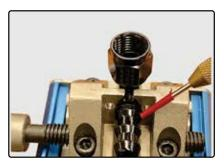
If the fitting is still pointing upward, remove the plastic inserts and use your free hand to guide the hose on.
