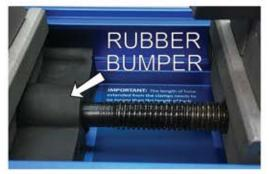
STOP IMMEDIATELY if the hose stops before it is fully installed. Check to see if the hose carriage is against the bumper.
